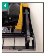
Remove belt from motor shaft and brush roll.
